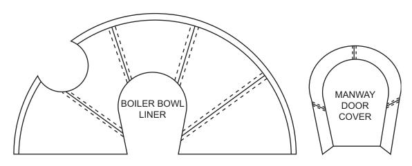
Simply install the liner inside the boiler bowl, in close contact with the boiler surface. Trim to accommodate protrusions, with a knife, if necessary. Inspect and clean out boiler, removing all loose debris, roll up and extract liner with attached metal filings.
